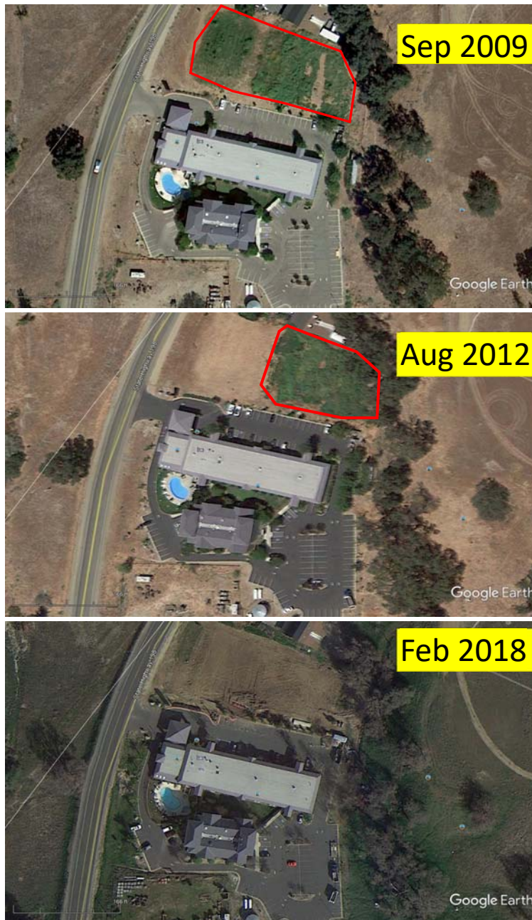
Figure 1. Google Earth images of the Three Rivers Comfort Inn from 2009, 2012 and 2018. In 2009 and 2012, note that septic effluent is surfacing and keeping the vegetation green north of the hotel. In 2018, note the grading and filling of the leach field and subsurface irrigation area.
